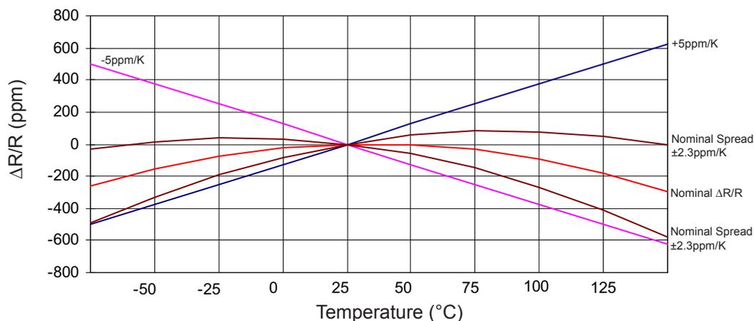
The TC adjustment is per charge at the reference temperature of 25°C ( $T_0$ ).
