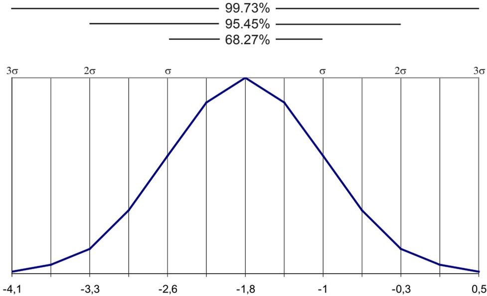
For a reduced temperature range from 0...60°C the nominal TCs are -0.6 ppm/K / +0.6 ppm/K and the nominal spread (3σ-area) of one charge is at ±2.5 ppm/K.
