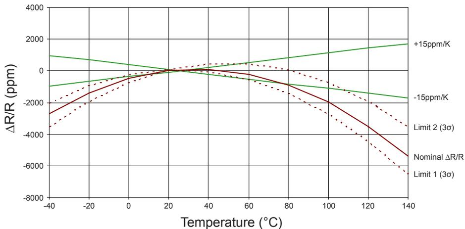
The  $dR/R(T)$ -curve of the precision-resistors series FPR, FHR and FNR as well as the precision-networks series FPN, FHN and FNN compared with the ultra-precision-resistor series USR/USN, UNR and UHR is more curved.
