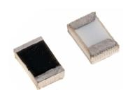
accurately measurable response, including t0.5 times from 0.1s to 3.3s, with dependable linearity and long-term stability. The halogen-free 0805 and 1206 SMD chip packages allow safe use where flammability is a risk. Standard nominal resistance values are  $100\Omega$ ,  $500\Omega$ , and  $1K\Omega$  for measurement current from 1.0mA to 7.0mA. Custom resistances are available to special order.
