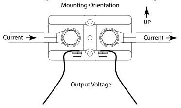
**Operating Current Derating:** For continuous operation, it is recommended that shunts are not run at more than two thirds (2/3) the rated current under normal conditions per IEEE standards for DC instrument shunts. At ambient temperatures above 40°C, the current must be further derated to prevent damage.
